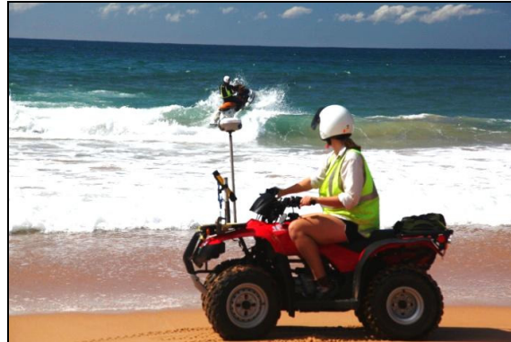
Figure 3 RTK-GPS beach survey and Jetski bathymetric surveying underway at Narrabeen-Collaroy.
